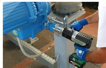
APB/APS tool on DREHMO Electric Actuator
